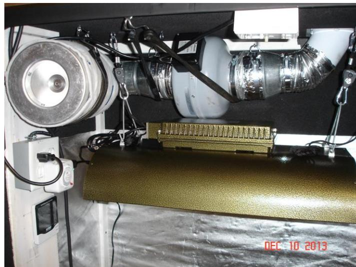
From left to right, a humidifier, an air “scrubber” (fan + charcoal filter to absorb any smells not caught by the first filter inside the cabinet), and on the right a [UV equipped HEPA filter](#) to take care of any dust, stray spores or mold.
